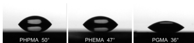
Figure 3. Static water contact angles determined at 20 °C for three hydroxyl-functional brushes: PHPMA (12 nm thickness), PHEMA (17 nm thickness), and PGMA (13 nm thickness).
